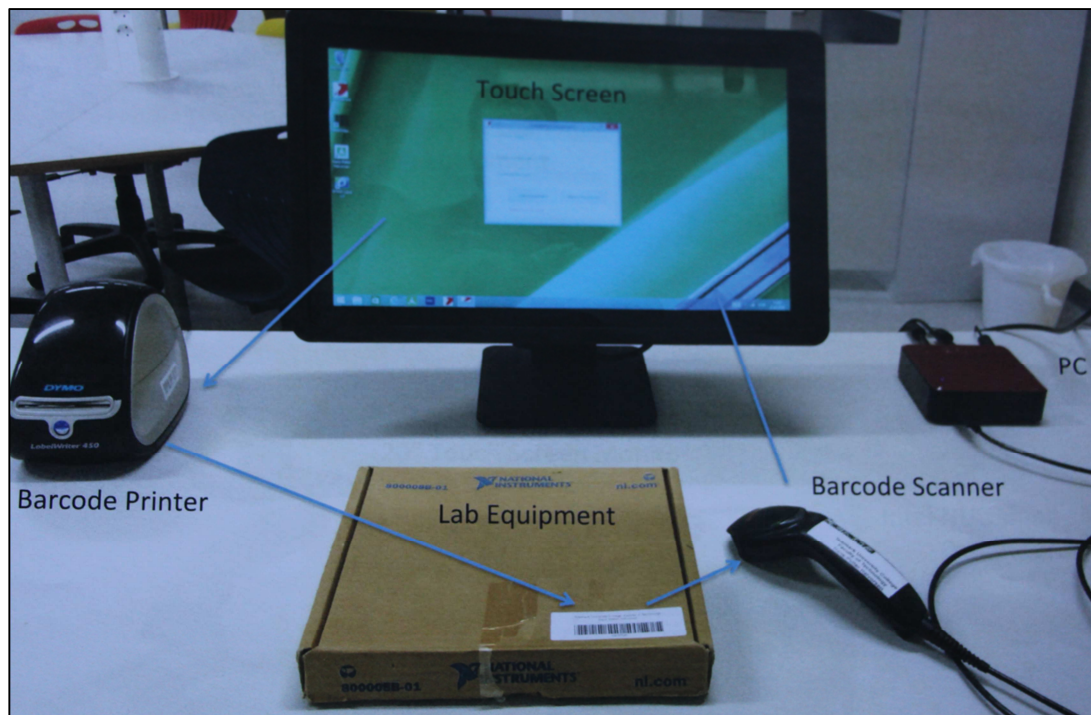
Figure 7-2 Lab Inventory System Station
